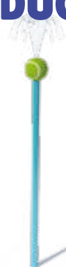
TENNIS BALL POST S-99.66 Dimension (inch/cm): h: 126" - 319 cm w: ø9.3" - ø24 cm Flow Rate: 8-15 gpm - 30-40 lpm Pressure: 8-15 psi - 0.5-1 bar Spray Zone (inch/cm): ø50" - ø127 cm
