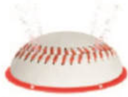
BASEBALL SPRAY S-02.23 Dimension (inch/cm): h: 16" - 40 cm w: 35.4" - 90 cm Flow Rate: 10-12 gpm - 36-48 lpm Pressure: 8-15 psi - 0.5-1 bar Spray Zone (inch/cm): ø83" - ø211 cm
