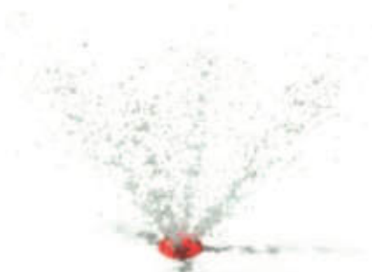
AQUA MIST S-05.07 Flow Rate: 9-18 gpm - 34-68 lpm Pressure: 4-8 psi - 0.3-0.5 bar Spray Zone (inch/cm): ø60" - ø152 cm
