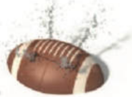
FOOTBALL SPRAY S-02.23.01 Dimension (inch/cm): h: 16" - 40 cm w: 44" - 110 cm Flow Rate: 10-12 gpm - 36-48 lpm Pressure: 8-15 psi - 0.5-1 bar Spray Zone (inch/cm): ø83" - ø211 cm
